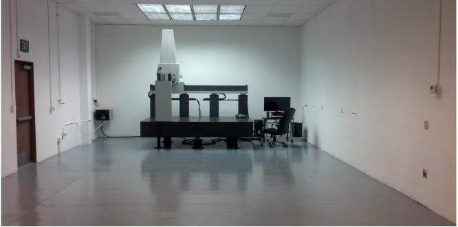
MY MACHINE, INC. INSTALLS a Coordinate Measurement Machine (CMM)
